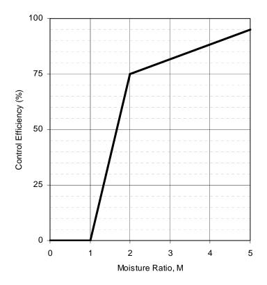
Figure 13.2.2-2. Watering control effectiveness for unpaved travel surfaces
